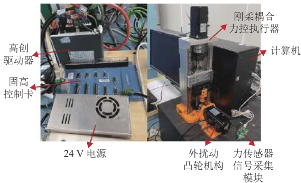
图 10 刚柔耦合力控执行器实验平台实物图 Fig.10 Experiment setup of rigid-flexible coupling force-control actuator
